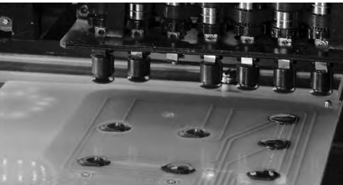
Automated Dome Placement
